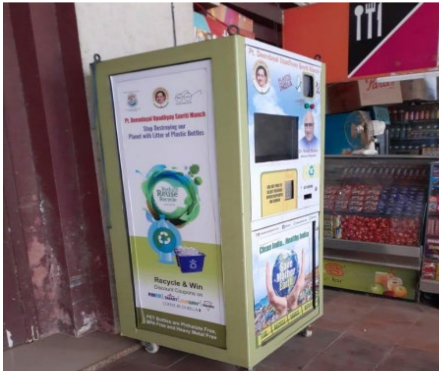
Plastic Bottle crushing Machine installed in the Canteen
